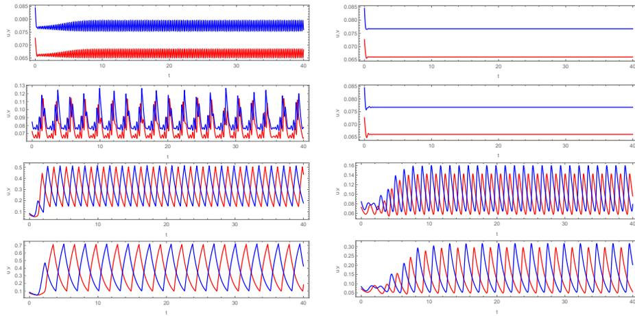
**Fig. 2.** Evolution of state variables  $u(t)$  and  $v(t)$  of system (2) with discrete time-delay (left) and strong Gamma kernel (right) for valued of the average time delay  $\tau \in \{0.07, 0.1, 0.5, 1\}$  (top to bottom). The values of the parameters are fixed:  $\theta_u = 0.1$ ,  $\theta_v = 0.2$ ,  $a = d = -6$ ,  $b = c = 3$  and  $\delta = 40$ . The same initial condition has been chosen in a neighborhood of the equilibrium.
