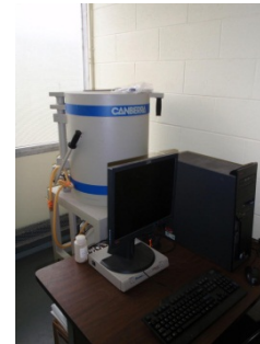
Fig. 3 Canberra BE2020 Germanium Detector housed at MSU for radionuclide measurement.
