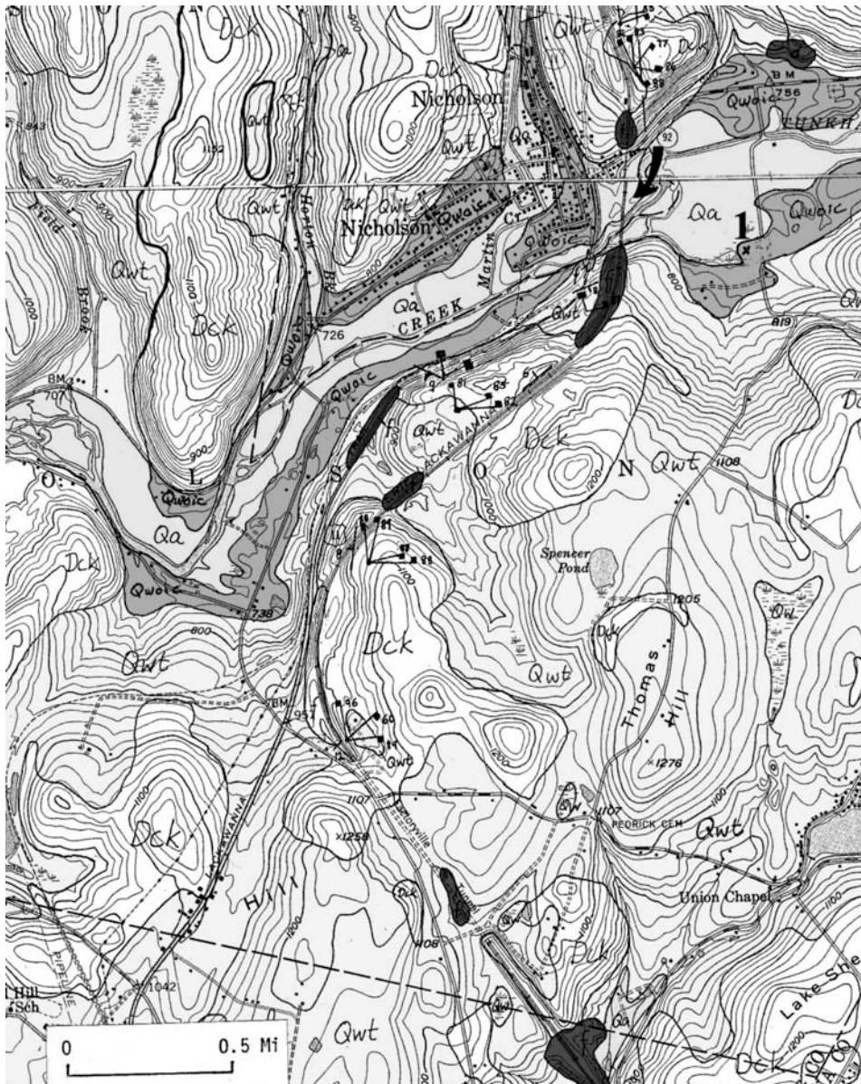
Figure 60. STOP 11 Location and Geologic map of the region around the Tunkhannock Viaduct (large arrow). Note the numerous deep cuts and fills—as well as the Nicholson (Factoryville) Tunnel—on the labeled Erie-Lackawanna grade (part of the “Summit Cutoff” of the old DL&W. (surficial geology after Braun, manuscript map).
