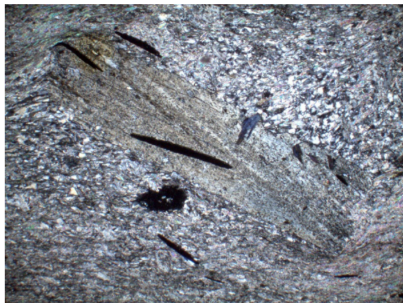
Figure 14. Thin section showing rotated chloritoid in schist from Stop 4. Top to right shear is shown by: high phyllosilicate density at top left and bottom right, corresponding low density at top right and bottom left, rotation of an early overgrown foliation, and by bent ilmenite grain (top left). Field width 3.67 mm, CPL.
