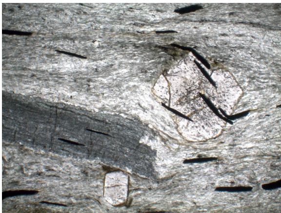
Figure 13. Thin section of chloritoid (center left) garnet schist from Stop 4. Top to right shear is shown by higher phyllosilicate density at top left and bottom right of garnet, and by bent ilmenite grains (opaque). Field width 3.67 mm, PPL.
