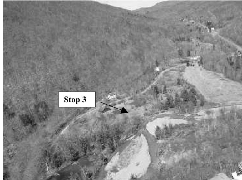
Figure 14. Aerial view of meander bend along Esopus Creek undergoing failure at Stop 3. Photo taken April 10, 2005. From NYC DEP et al., 2007.
