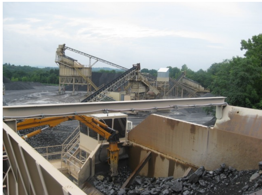
Figure 19. Photo showing feed hopper of primary crusher at aggregate processing plant at the Colarusso quarry on Becraft Mountain.
